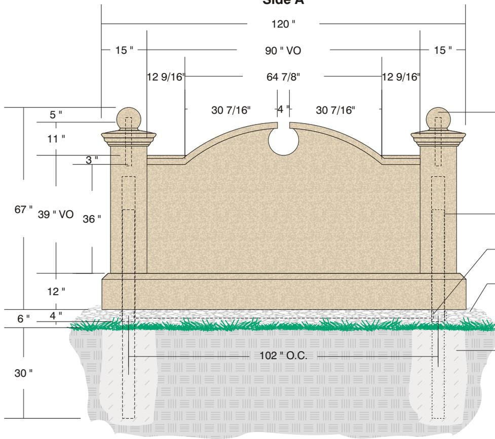
DeSign Stone sign system with (2) 4 1/8" x 4 1/8" x 48" full round internal mounting sleeves, (1) 12" x 120" x 18" base, (1) 48" x 93" x 9" body, (2) 42" x 12" x 12" columns, (2) 5 1/8" x 18" x 18" column caps, (2) 7" x 8" x 8" ball caps with (2) 2" x 2" x 16" full round posts for ball cap stability, and (2) 14" x 44 1/2" x 12" body caps
